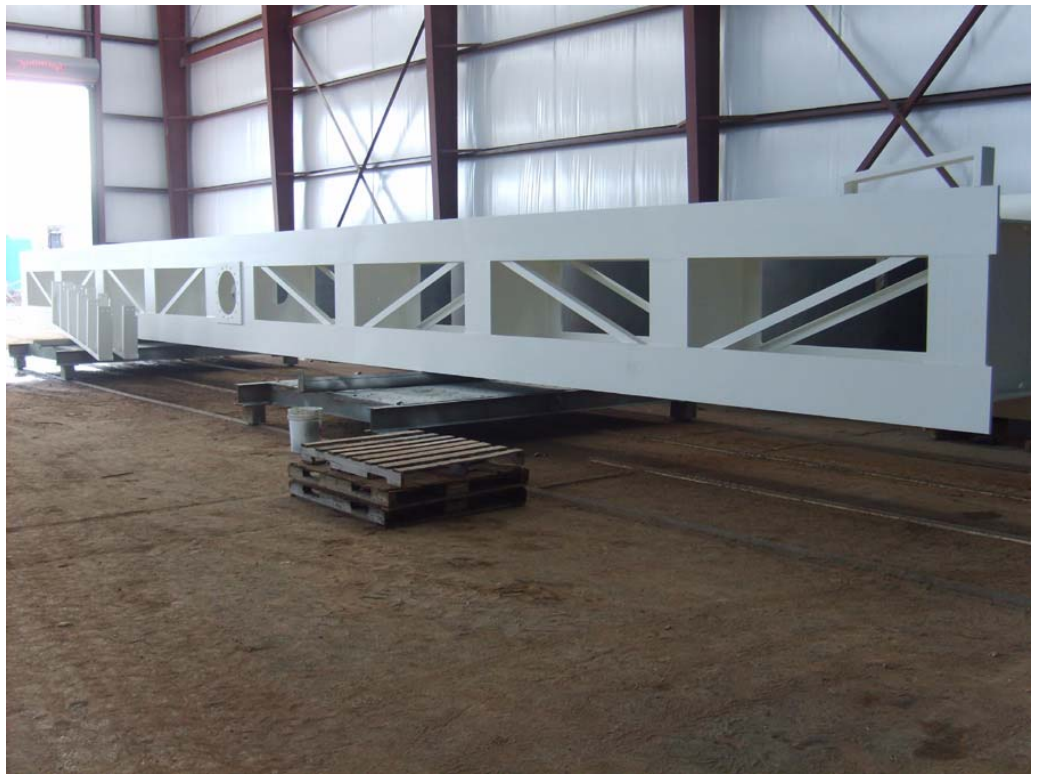
Large Scale – 60 Foot Mixing Support For Open-top Tank
