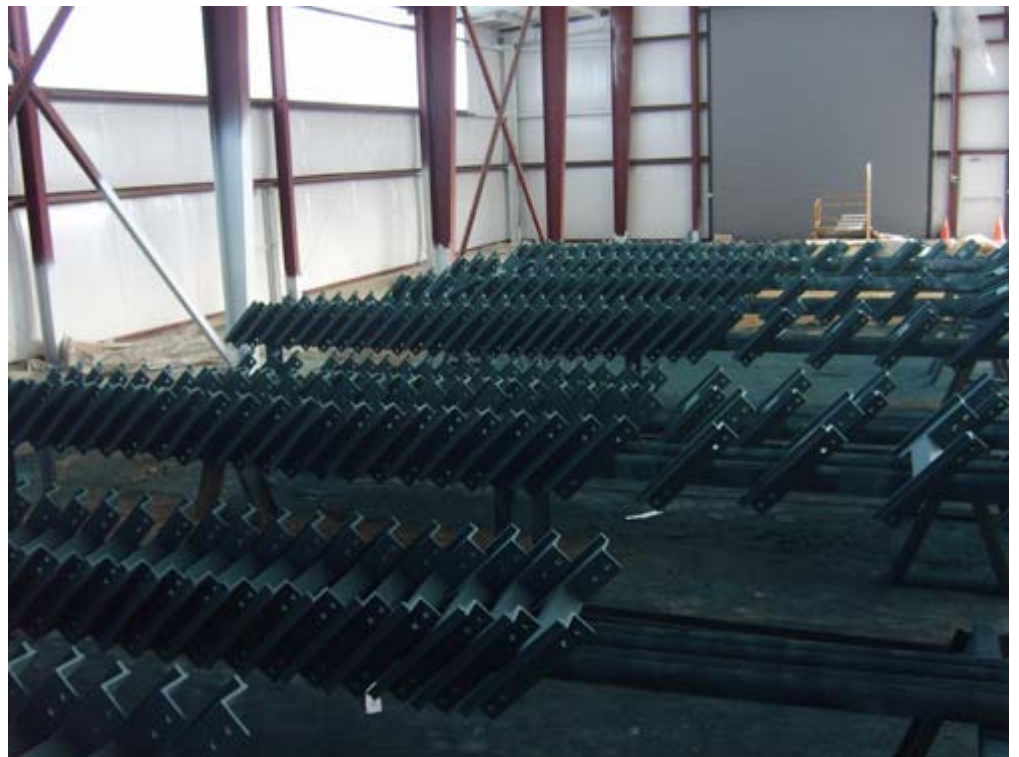
High volume – H Brackets after coating application
